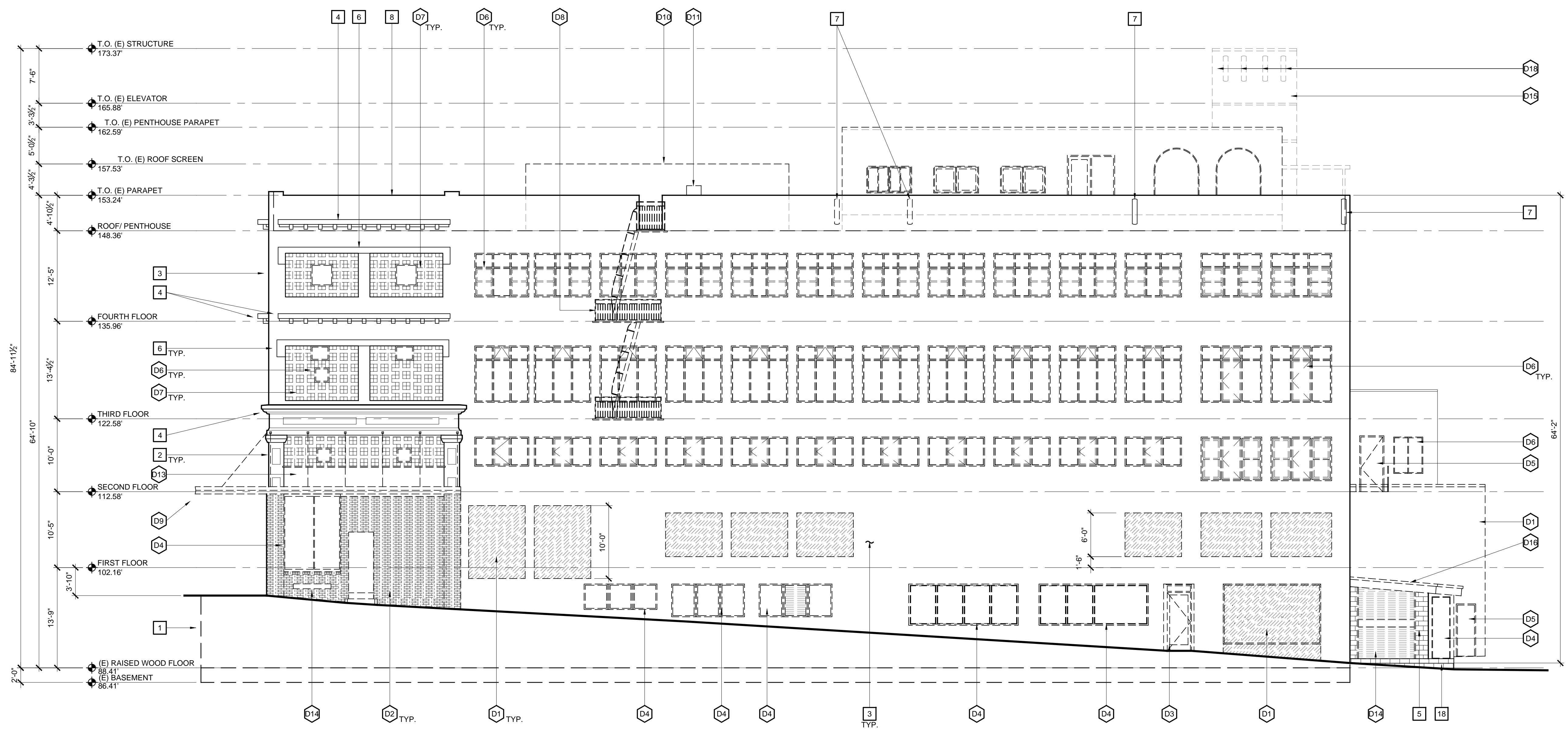
1 EXISTING/DEMOLITION EAST ELEVATION SCALE: 1/8" = 1'-0"
